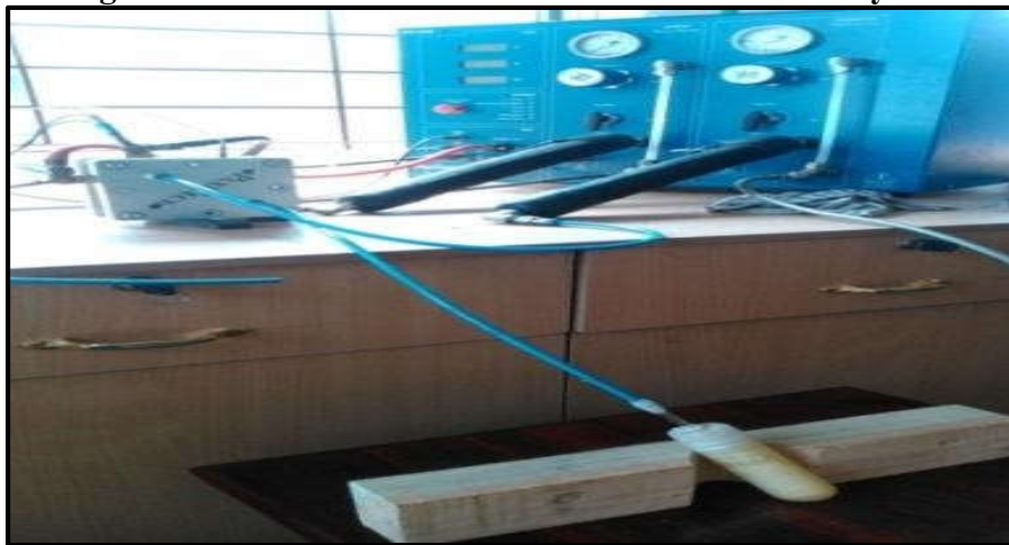
Figure No.4: Assembled fuel cell with CaCl2 connected at the outlet
