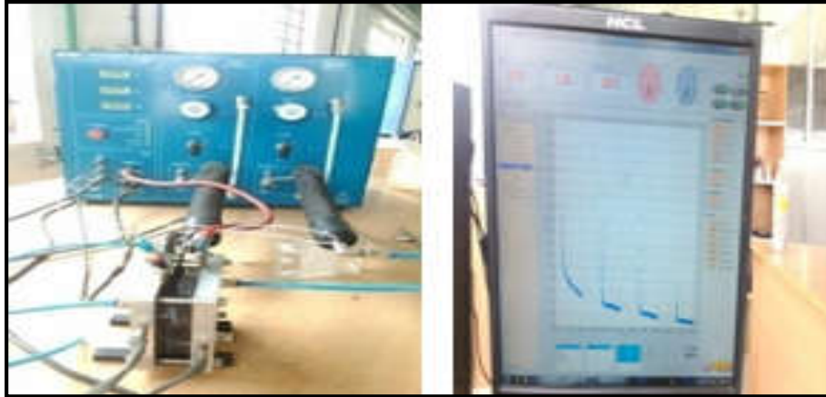
Figure No.3: Interfaced fuel cell test station and the system
